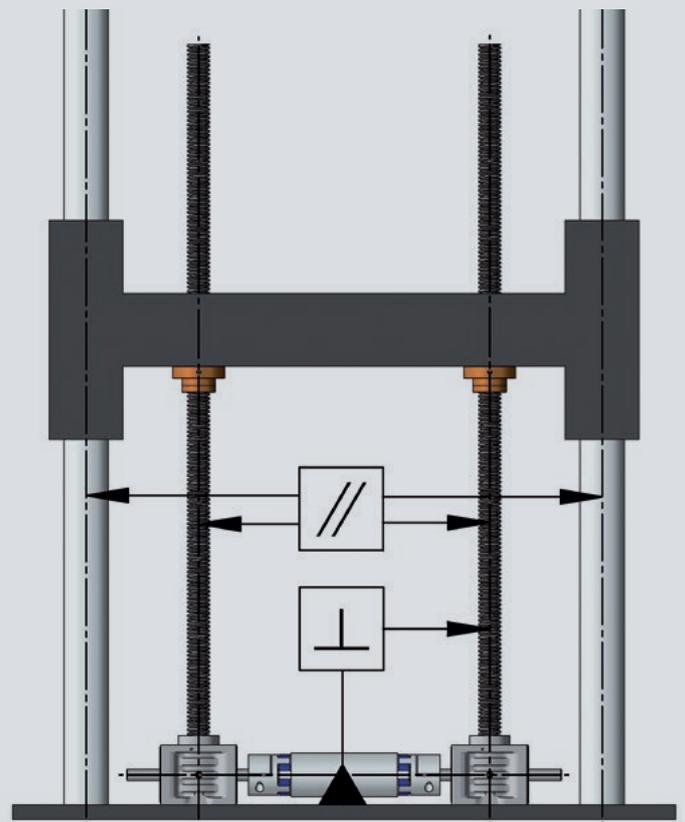
the guides must be guaranteed, otherwise, the system can get stuck during operation. Also, the fastening surfaces of the gearbox must be exactly at right angles to the guides, otherwise jamming can occur. This results in faster wear and/or destruction. Basically, mounting surfaces for the nuts must also be at an angle. To save time and costs in this respect, the compensating nuts can be used. Another possibility of balancing out certain inaccuracies in the design is the use of Cardan adapters.
